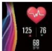
4.1 The heart rate sensor shall be closely attached to and well contacted with skin in measurement of heart rate. If the smart bracelet is too loose, the sensor light will expose, which can result in inaccurate measurement. It is prohibited to look steadily at the green light of sensor; otherwise, it may make eyes uncomfortable.
